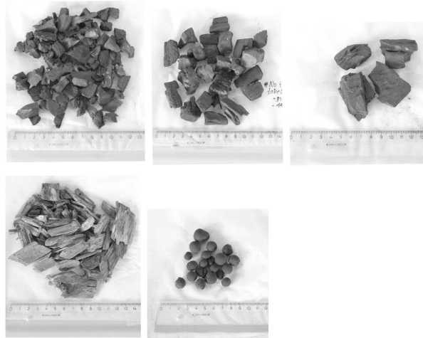
Figure 4.3: Some of the used fuels. Upper left to right: small char (10 – 15mm), medium char (15 – 30mm), large char (30 – 40mm). Lower left to right: wood chips (10 – 40mm), stones (10mm).
