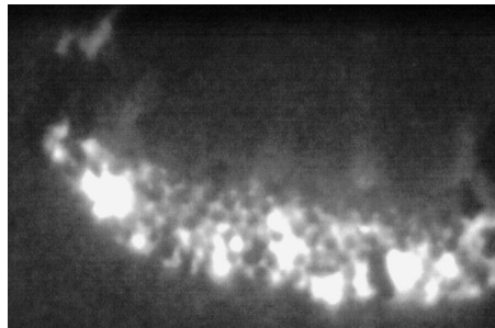
(b) \text{OH}^* chemiluminescence image of the ignition front.
